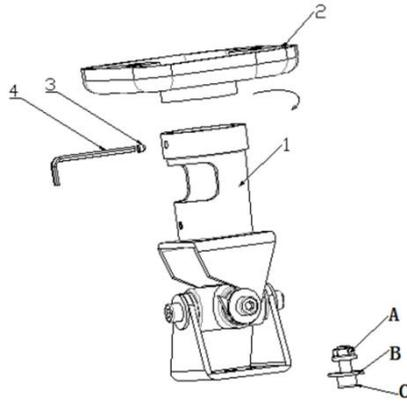
2. To install the laser units, connect the laser unit together with the hold A, B and C. After adjust the direction and position, fix the screw with 6mm hexagon bar wrench. figure 1 for expansion screws, which used for fixed on the wall. The angle adjustment range as shown below sketch:
