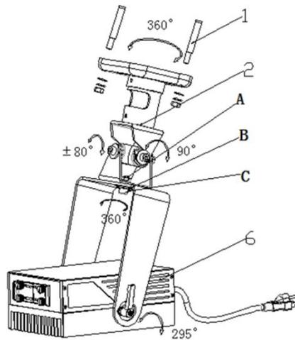
3. Beam aperture shutter: Loose the screw (No. 2), then the shutter can be moved and adjustable.
