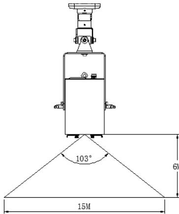
The Vertical downward projection angle is about  $103^\circ$
