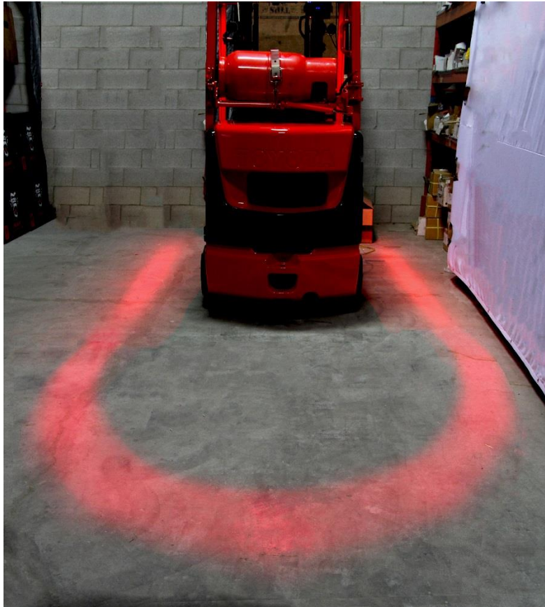
Forklift Arch Light shown in combination with two forklift red zone lights (must be purchased separately)
